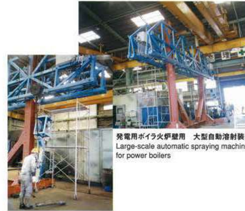
発電用ボイラ炉壁 自動溶射装置による現地溶射施工 On site spraying for the boiler tubes of the power station using the automatic spraying machine
