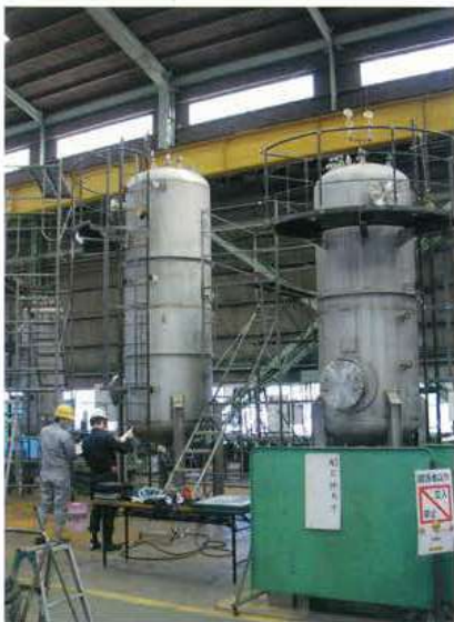
消防法SUSタンク 耐圧検査状況 The stainless steel tanks under pressure test according to Japanese fire protection law
