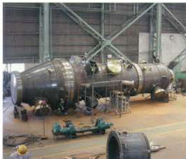
高圧ガス保安法 高圧ガス容器製作 Manufacturing a gasification furnace according to Japanese high pressure vessel code
