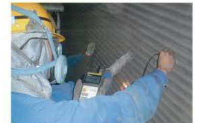
溶射膜厚検査 Inspecting thickness of the coating
