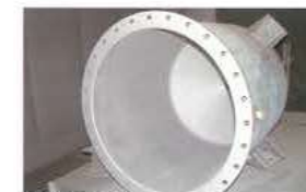
タンク内面溶射 Wire spraying for inner surface of the cylindrical tank
